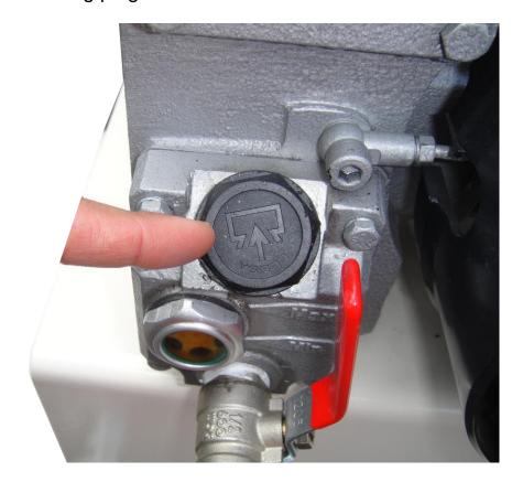
**Step 3**: Open the unloading valve (offloading oil).
