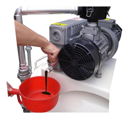
Step 4: Change the oil filter. (EUROVAC\_F100) (After changing, please refill the SAE 30 or 40 motor oil which is non-detergent about 1liter)
