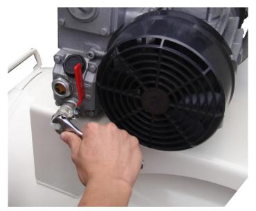
Step 2: Remove the oil filling plug
