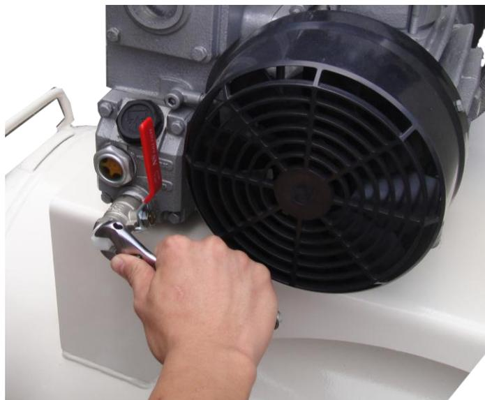
**Step 2 : Remove the oil filling plug**
