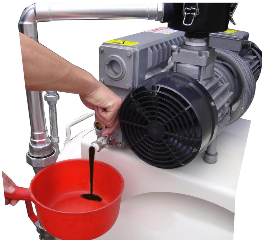
**Step 4 :** Change the oil filter. (EUROVAC\_F100) (After changing, please refill the SAE 30 or 40 motor oil which is non-detergent about 1liter )
